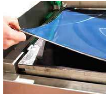
Magnetic sticky table is easy to replace
