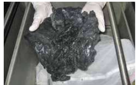
Washed photopolymer residues are caught in the filter and a solid polymer cake remains
