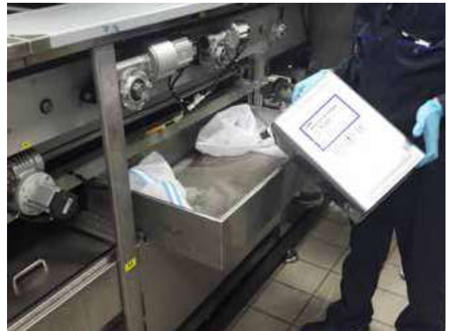
Operator friendly roll-out tank system for easy access
