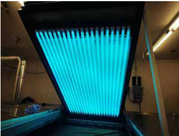
Inline-UV post-exposure ensures high plate uniformity
