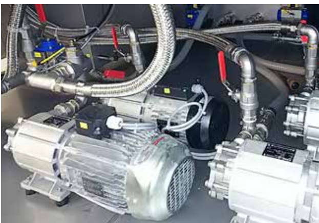
Magnetic stainless steel pumps for easy maintenance. This pump type does not have a gasket, meaning there is no problem with water leakage
