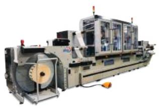
Converting systems for RFID production vary considerably from client to client. The Omega converting line gives customers a wide variety of functions and features to choose from in order to build a converting system that meets with their individual requirements. Converting modules are available in 330mm (13"), 430mm (17") and 530mm (21") web widths and can produce self-adhesive label solutions as well as tag and ticket products.
